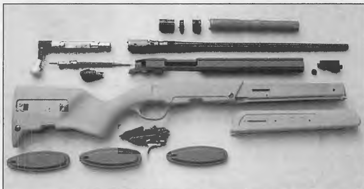
Steyr Scout rifle completely disassembled and shown with three buttstock spacers and the armorer's wrench used to remove the barrel from the receiver.
